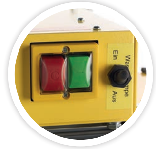
Disengageable water pump for dry run
