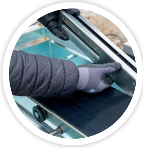
Interchangeable suction channel for easy adaptation without tools (patented)
