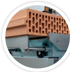
Telescopic platform extension for larger materials
