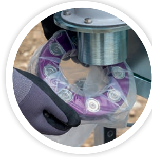
Magnetic holder for to replace the dust bag in seconds
